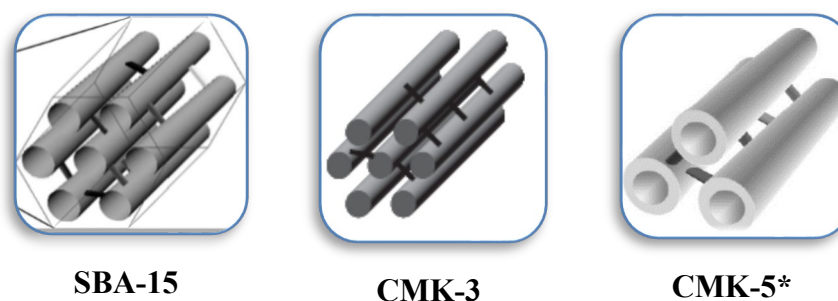
Figure 4. Scheme of some porous structures of ONC from SBA-15.* Reproduced with permission from reference [23].
