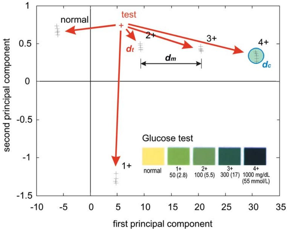
**Fig. 5.** Principal components plot of the different pads in the calibration label of a Glucose tests for urine samples. A potential test result is indicated as “test” together with the most relevant distances for classification purposes.  $d_t$  minimum distance to a reference spot,  $d_m$  mismatch distance and  $d_c$  calibration distance (i.e. maximum spread of calibration points for a given classification) [17]
