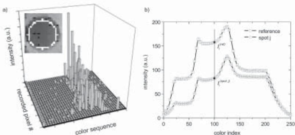
**Fig. 2.** a) Intensity distribution of each pixel composing the recorded image of a single spot along the illuminating sequence. b) Transmitted intensity features obtained as the average and standard deviation of all the pixels involved in the image of each well (spot  $j$ ) for each color  $i$  of the illuminating sequence. Results are shown for a reference blank spot and a red one. (In the example the color sequence contained 250 different indices).
