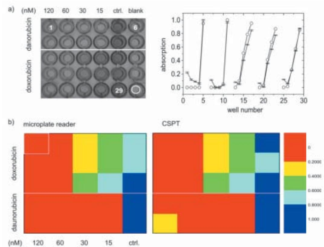
**Fig. 3.** Comparison between a cell viability test monitored by a normal microplate reader and CSPT [3]. a) Picture of the array used for the analysis (a total of 30 wells) and the absorption measured by both methods (open circles for the reference technique and error bars for CSPT).
