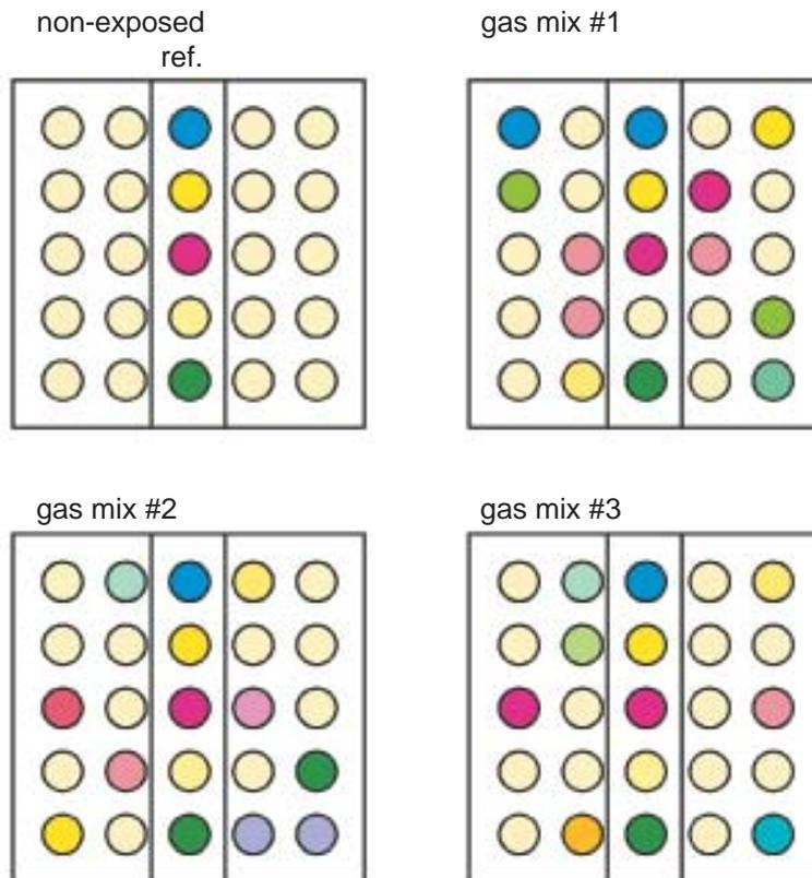
*Fig 6. Schematics of an electronic nose application of CSPT.*
