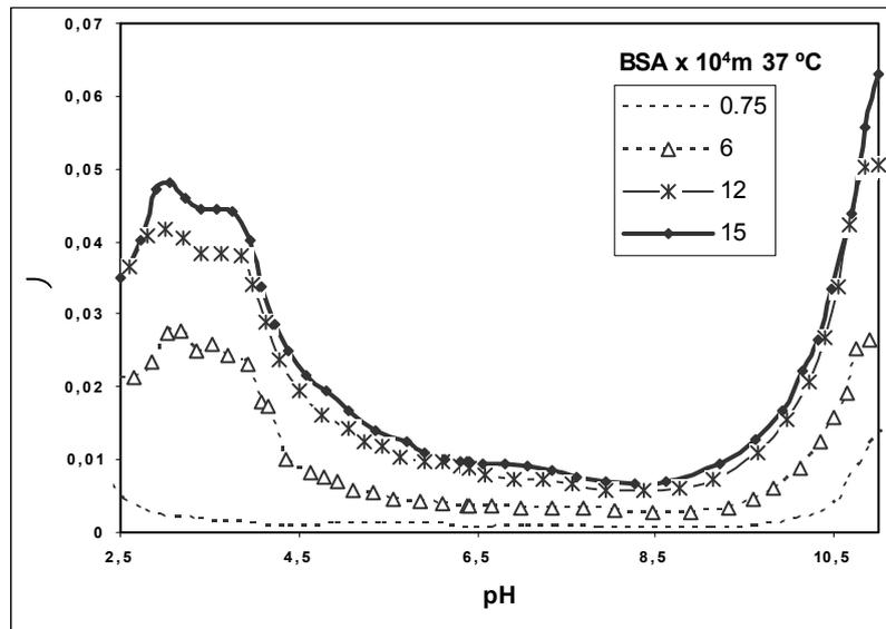
**Figure 2.** Buffer capacity at different pH values. BSA solutions 0.75 and 15 x 10<sup>-4</sup> molal at 37 °C.
