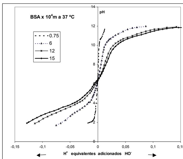
**Figure 1.** Potentiometric titration of BSA. Concentrations from 0.75 to  $15 \times 10^{-4}$  molal at 37 °C. Acid (or base) equivalents added in function of pH.
