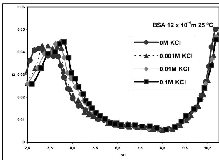
**Figure 3.** Buffer capacity in function of pH. Effect of the addition of KCl 0.1, 0.01 and 0.001M at 25 °C.
